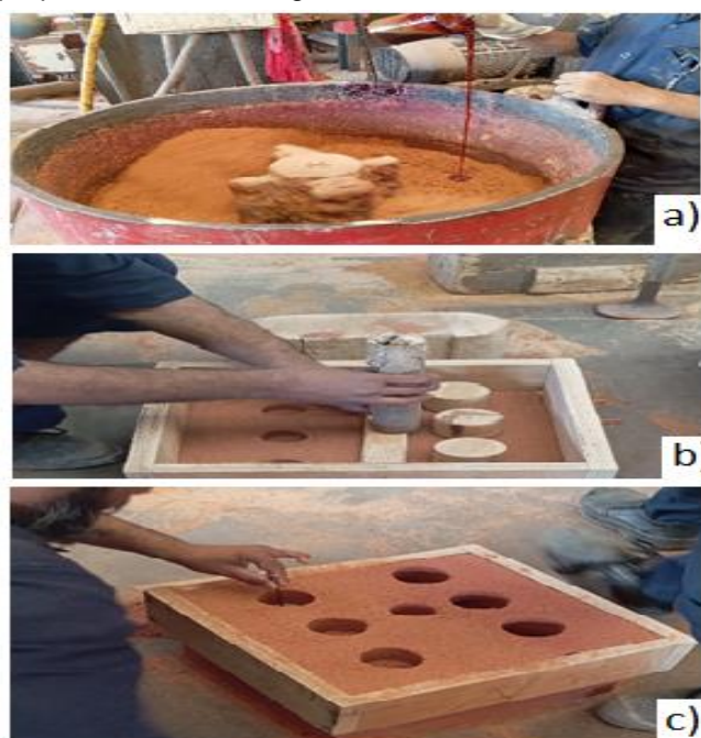
Figure 1: Alpha set sand mold/core preparation a) Mixing of sand with alpha set b) Making sprue and runner c) Cope and Drag
