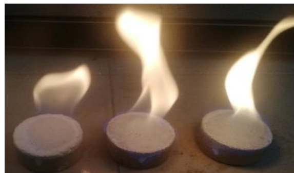
Figure 7: Flame ignition of alcohol-based zircon coating on sand mold
