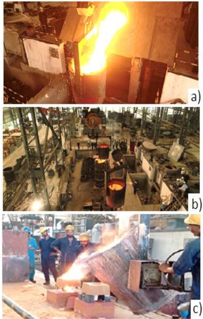
Figure 3: Melting of Steel for casting a) pouring of molten metal from furnace to crucible b) transferring of molten metal c) pouring of molten metal to molds
