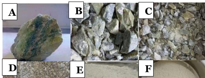
Figure 1: Picture of lizardite before heat activation , (A): Lizardite in rock form, (B): small pieces of lizardite after hammering , (C): After Jaw crusher , (D): After Blake jaw crusher ,(E): After ball mill ,(F): After sieve analysis
