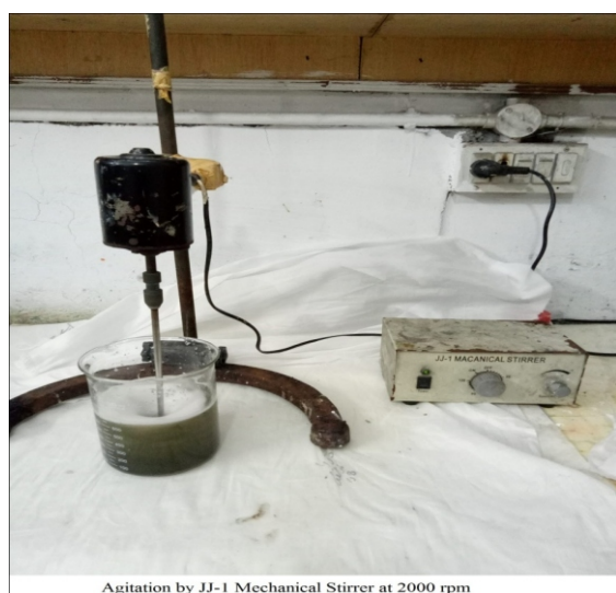
Agitation by JJ-1 Mechanical Stirrer at 2000 rpm
