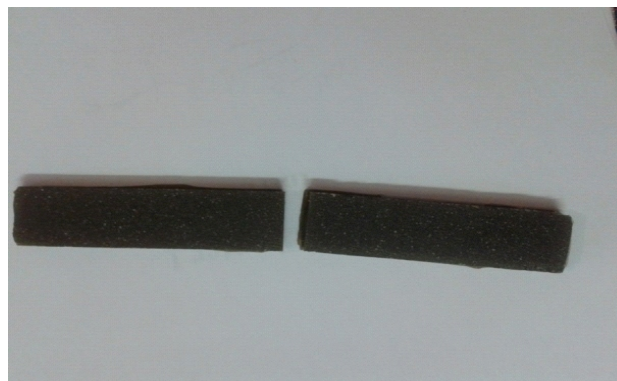
Figure 3: Flexural testing sample after fracture
