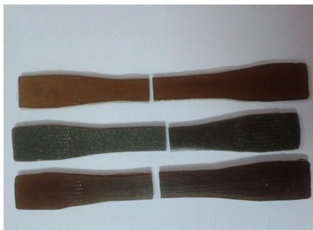
Figure 2: Tensile testing after fracture
