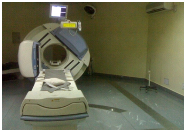
Fig. 1. The setup for flood uniformity test of gamma camera Infinia Hawkeye 4 (GE Health Care U.K)
