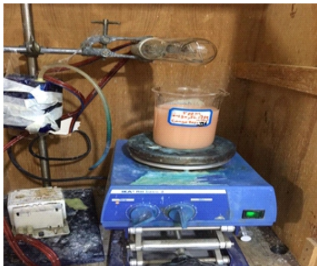
Figure. (3): Real image for (a) the reactor system without using UV-lamp, and (b) photo-degradation surface.
