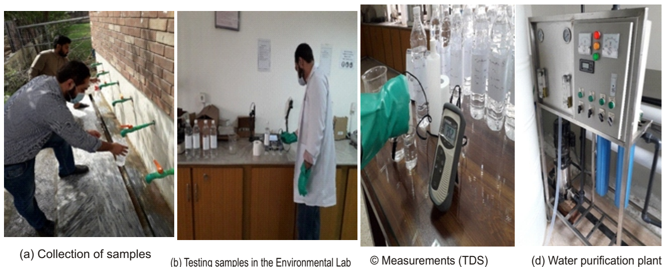
Figure 1: sampling & testing of water from water purification plants (a) Collection of samples (b) Testing samples in the environmental lab (c) TDS measurements, and (d) Water purification plant
