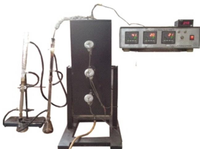
**Figure 1:** *Three zone Tube Furnace*
